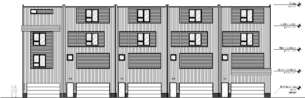
3 BUILDING 2 - SOUTH ELEVATION SCALE: 1/8" = 1'-0"
