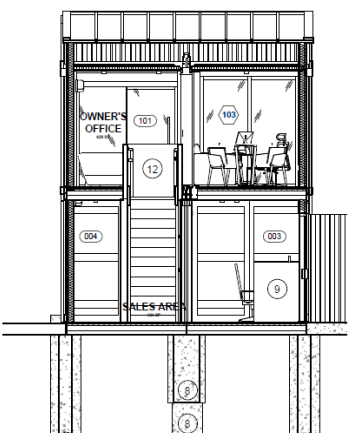
5 SOUTH-WEST SECTION A3.0 SCALE 1/4" = 1'-0"
