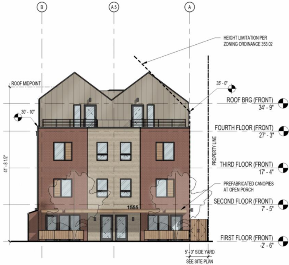
1 WEST EXTERIOR ELEVATION 3/32" = 1'-0"
