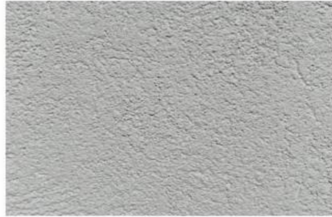
PT-4 5/8" SOFFIT STUCCO W/ SAND FINE FINISH; BENJAMIN MOORE STORMY MONDAY (MATCH EPS-1)
