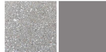
CONCRETE TYPE 1 - LIGHT SANDBLAST FINISH
